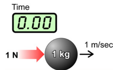
Figure 2.9: The definition of a newton.
